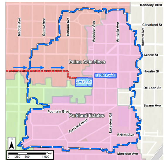
Figure 3-11 – Cleveland Street Outfall System – Actual High Flow Conditions (Negative Flow)
